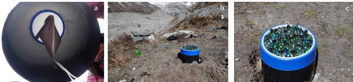
Figure 5: Dust collector installation. a: Filter bag inside dust collector, b: Dust collector placed in the field, c: Marbles in the funnel of the dust collector
