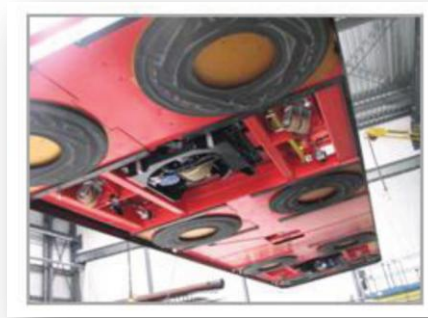
Figure 24: Air casters as conceived to propel the HTS using air pressure to 'fly' as a hovercraft.
