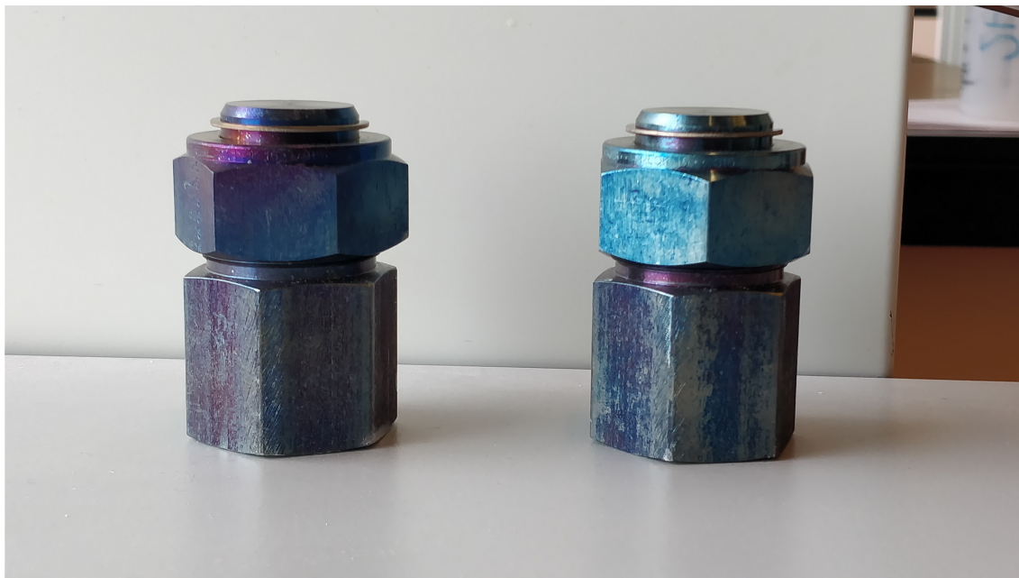
FIGURE A.1: Photographic image of stainless steel reactors used for air-tight melt-infiltration of \text{NaBH}_4 under \text{H}_2 pressure.
