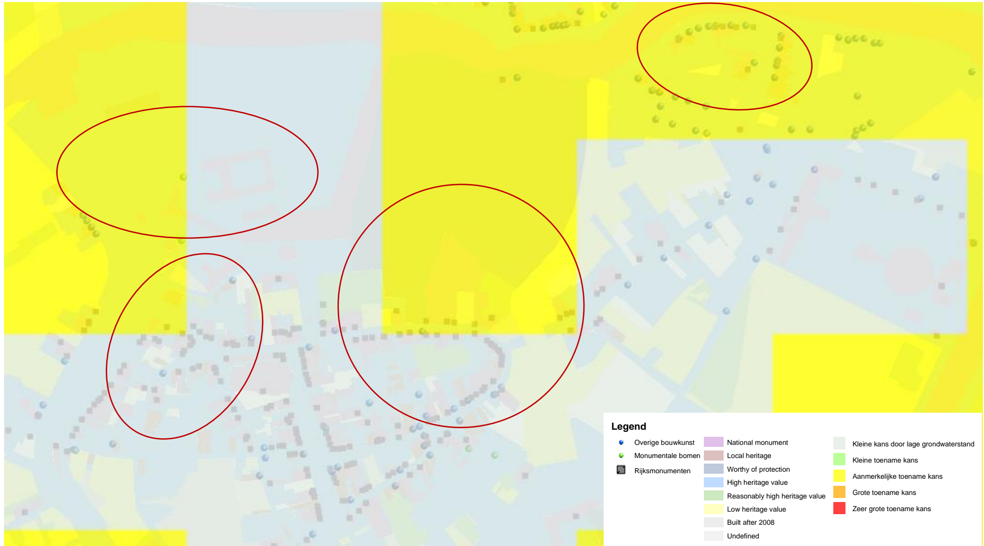
Figure 34 - Potential groundwater nuisance in 2050 WH superimposed on Breda cultural-historic value map (Northern rectangle) the tiny purple squares are nationally listed monuments, the green dots are monumental trees, and the blue dots are municipal listed buildings (1:4.500)
