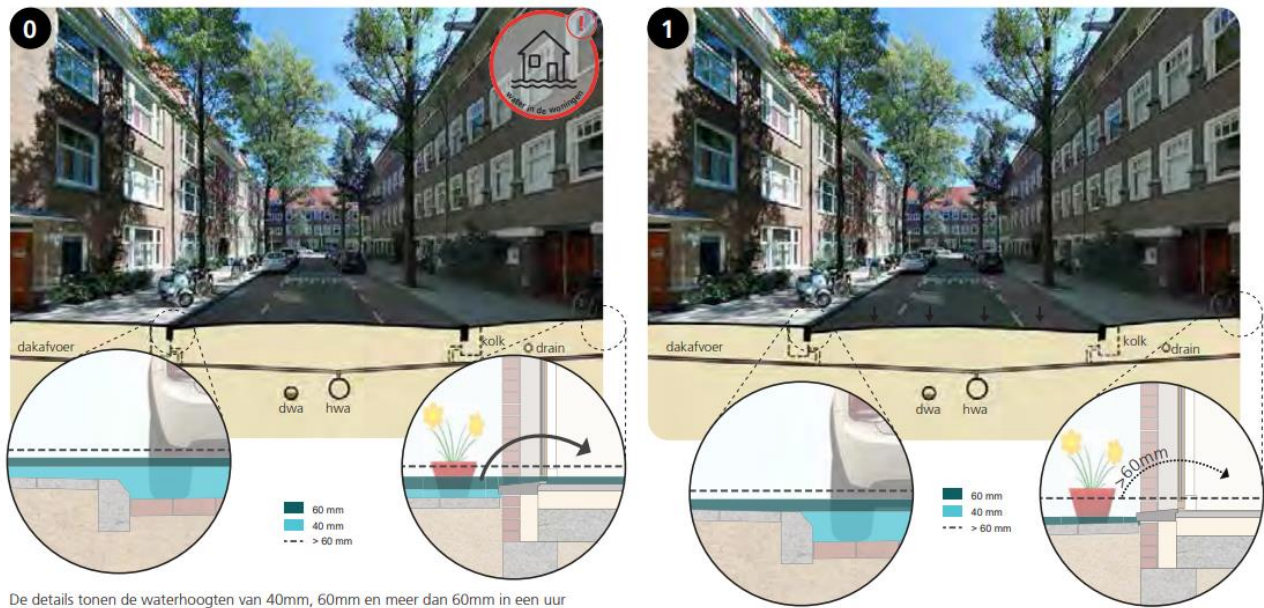
Figure 16 - Comparison traditional renovation option 0 and collection at street level option 1 (Kluck et al., 2017, 28)
