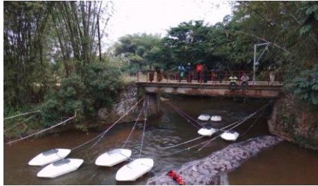
Figure 14 Photo showing the use of micro-hydro turbines at a pilot project in the DRC (Source: Energies de la Mer)
