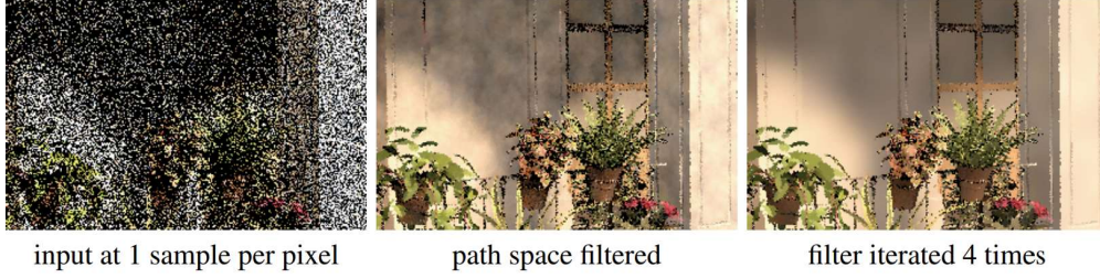
Figure 4: Iterated weighted averaging very efficiently smooths the solution by relaxation at the cost of losing some detail. Obviously, path space filtering brightens up the image by replacing black pixels of the input with the weighted averages. Model courtesy of G. M. Leal LLaaguno. Original image and caption reproduced with permission from Keller et al. [2].
