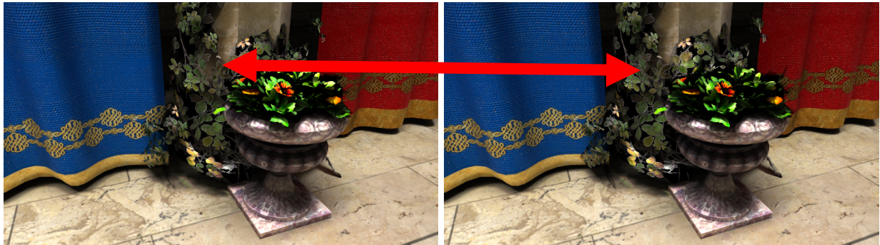
Figure 33. Sponza Close rendered with 1024 SPP using CUDA (left) and rendered using OpenCL (right). Note that some parts of the alpha textures are rendered different.
