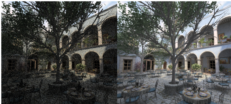
Figure 2. Images generated from path tracing with the difference in quality depending on the samples taken. The image on the left is generated with eight samples per pixel, and the image on the right is generated with 1024 samples per pixel [12].
