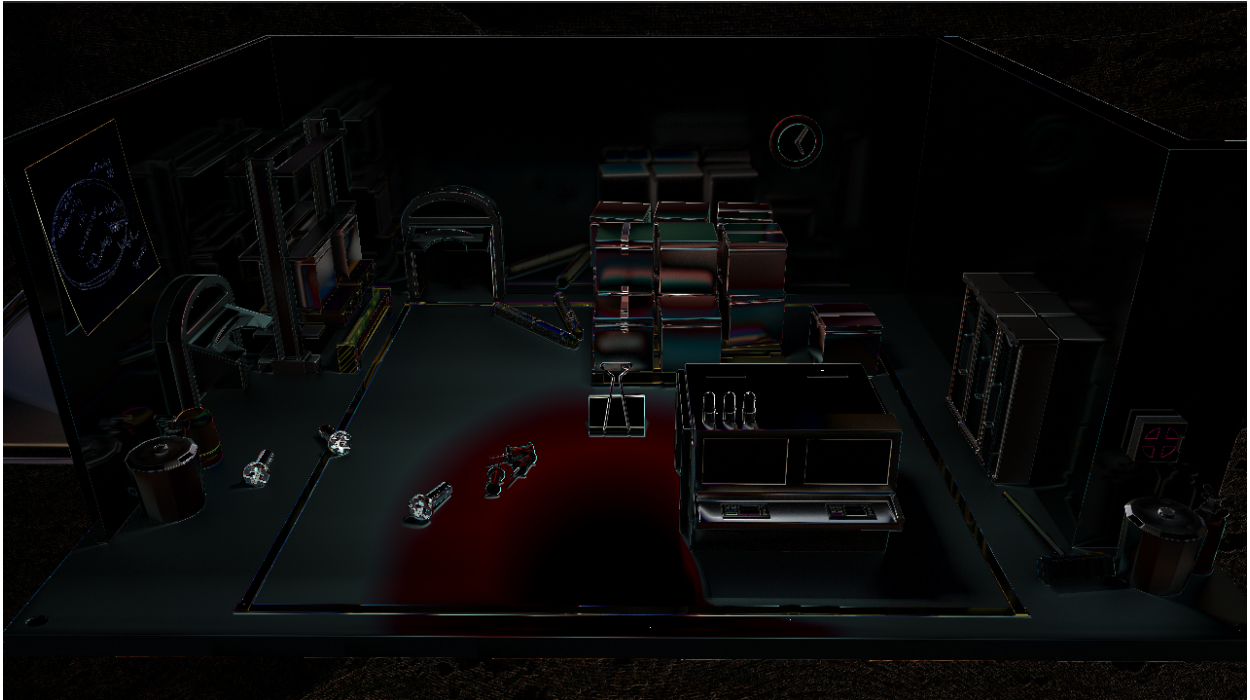
Figure 11: The image difference of the two rendering cores on the Pica Pica scene after collecting 1024 samples per pixel.
