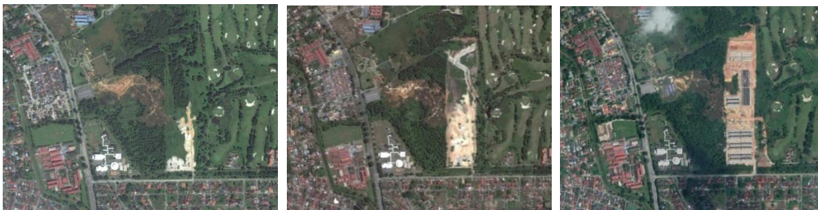
Figure 11: Visual comparison of time series maps to identify construction sites. Example of the progress of a building site in Ipoh during 2014, 2017 and 2019. Source: Google Earth (2014, 2017 and 2019).
