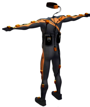
Figure 2.2: Xsens MVN consists of 17 inertial and magnetic sensor modules [54].
