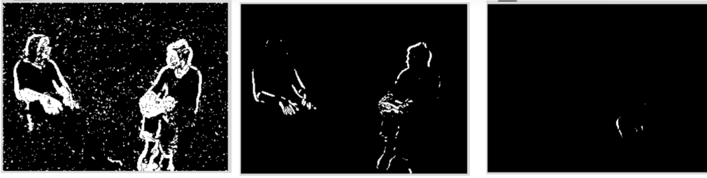
Figure 2.1: Removing noise from the measured movement by applying a threshold. The left image has a too low threshold, the center image has a good threshold and the right image has a too high threshold. This Figure is provided by [49].
