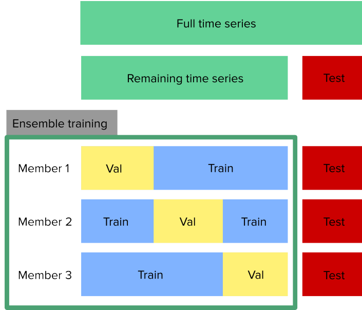
Figure 3.3: An illustration of the data splitting and ensemble training which is applied in this study. From a full time series, first the test data (red) set is split apart. The remaining series is then split into (here) three segments which are used to train an ensemble model. The ensemble members are trained on the training data set (blue) and hyperparameters are optimized for the validation data sets (yellow). The model ensemble that performs best in terms of the average loss on the validation data set is evaluated on the test data set.
