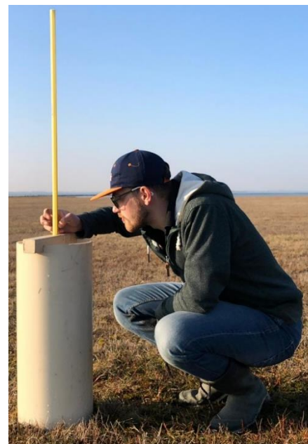
Figure 7, Side view infiltration test during the measurement
