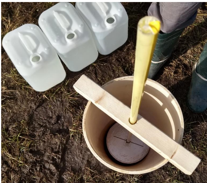
Figure 8, Infiltration test setup: Three jerry cans with saline water, tube, buoyant disk, holder and measuring stick
