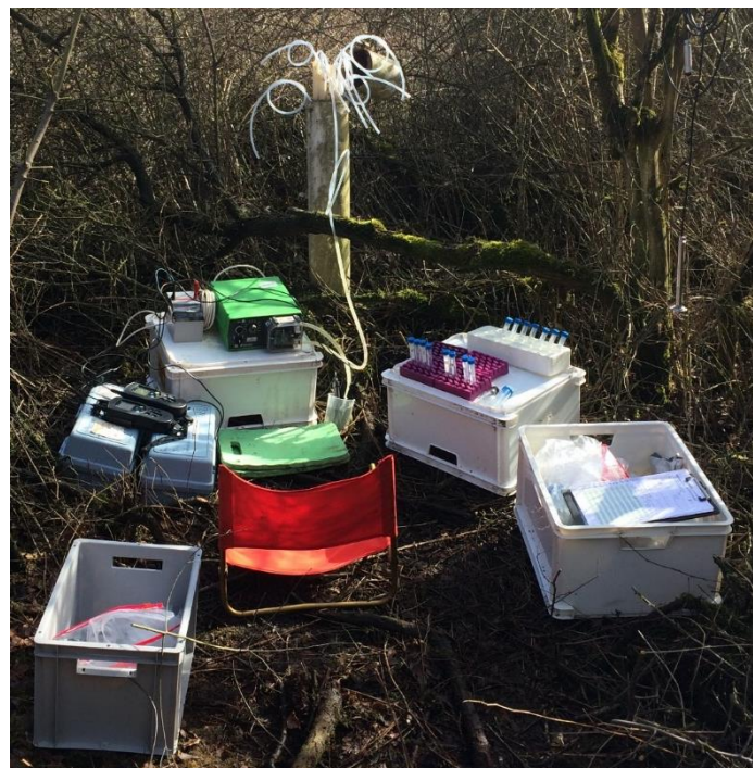
Figure 11, Field setup for the chemical sampling of the groundwater
