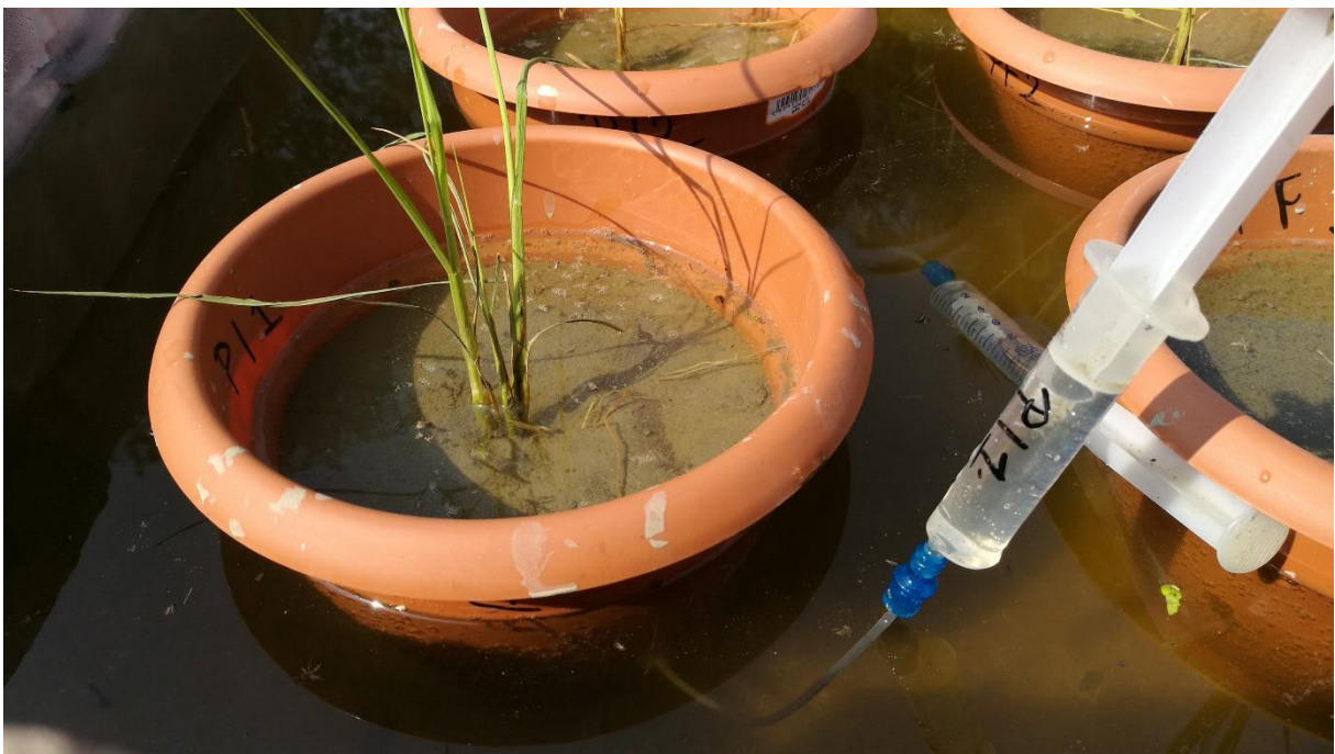
Figure 3.3 Pore water samplers attached to pots (own work)
