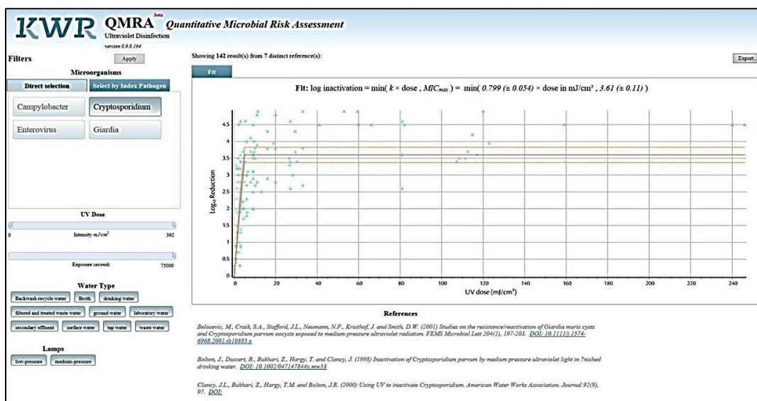
Figure 5: The log removal of Campylobacter using UV treatment through QMRA treatment calculator. Source: Watershare.eu.
