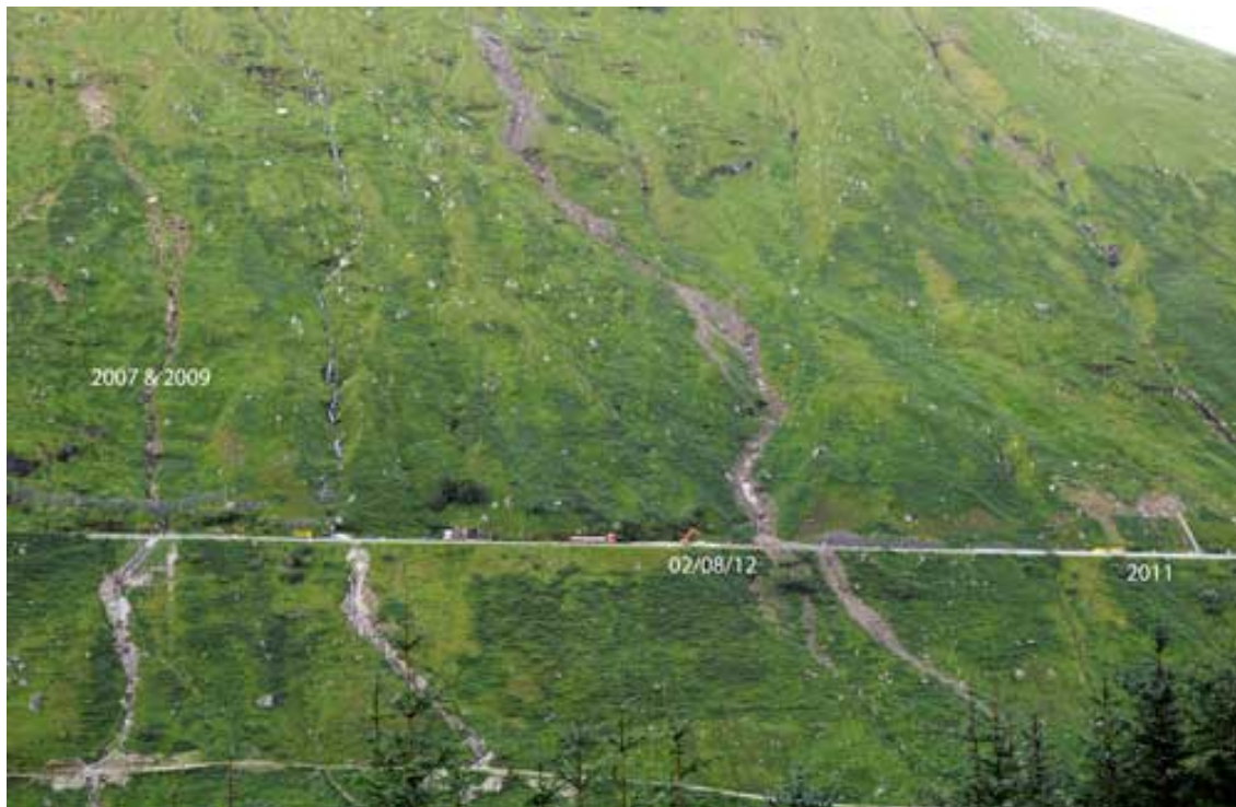
Figure 1: Rest and Be Thankful hillslope with indications of past mass movement flowpaths (BGS Landslide Team, 2018b).
