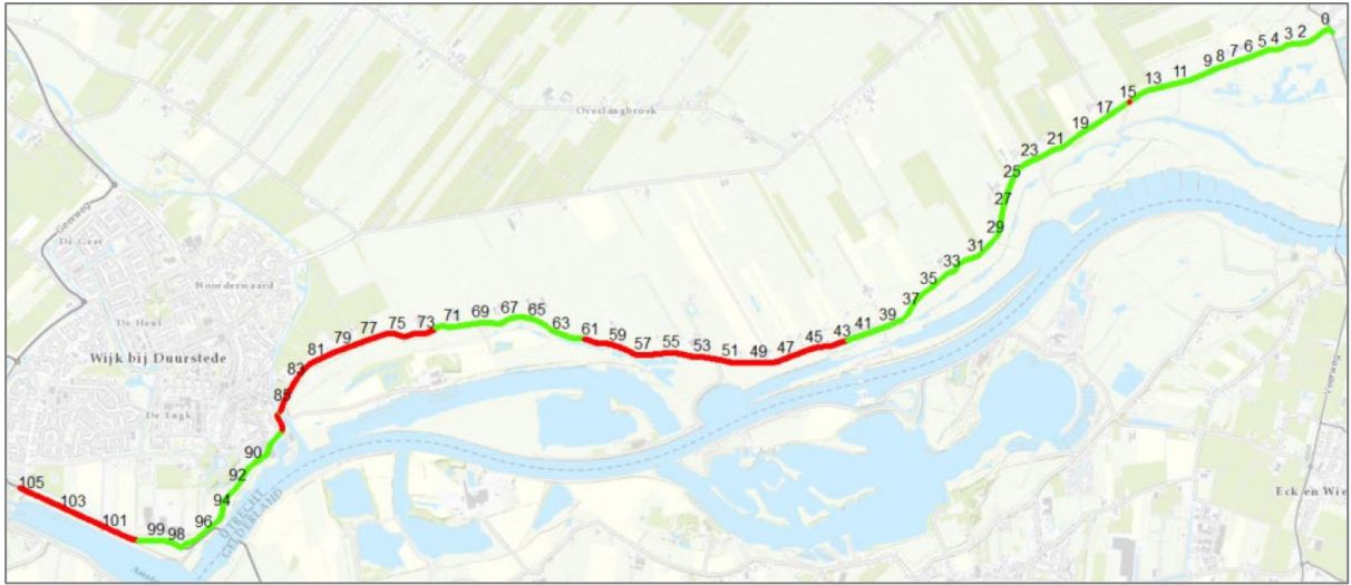
Figure 2.2: Inward macro-stability assessment of the WAM river dike for a normative high water level (numbers represent dike poles (DPs)).
