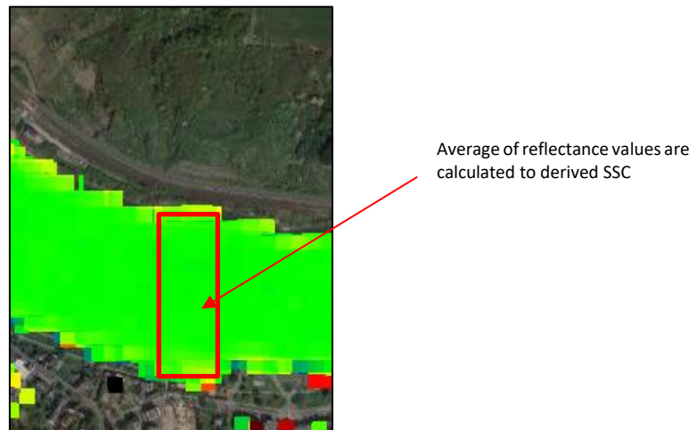
Fig. 2.5. Average of reflectance values are calculated to derive SSC
