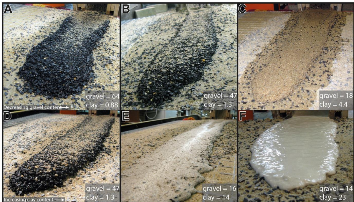
Figure 2.4. Depositional patterns of flow with decreasing gravel content (A-C) and increasing clay content (D-F) (after: de Haas et al., 2015)
