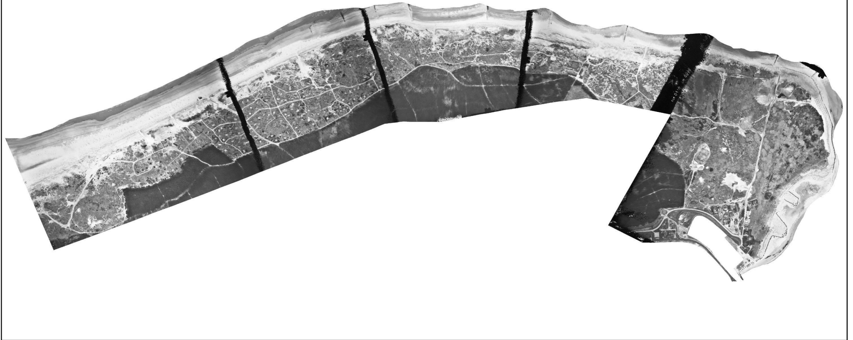
Figure F2: Orthophoto of the 1981 aerial photographs, made with the 1981 DEM-SGM.
