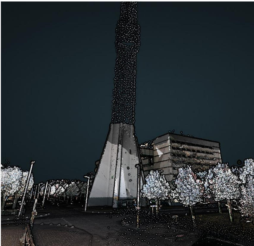
Figure 6.12: Overlay of MLS and ALS dataset in Pointer. The two datasets complement each other but also partially overlap (Source: Gemeente Rotterdam / own work)
