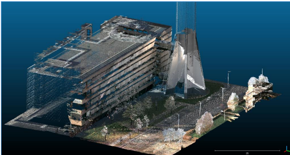
Figure 5.5: Overlay of different point clouds in CloudCompare (source: Gemeente Rotterdam / own work)
