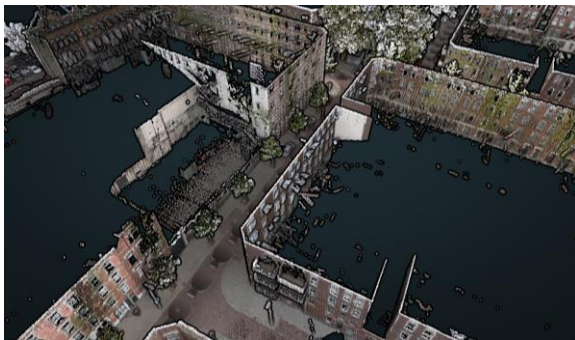
Figure 3.7: MLS: little roof top information of the Noordereiland (source: own work / Gemeente Rotterdam)
