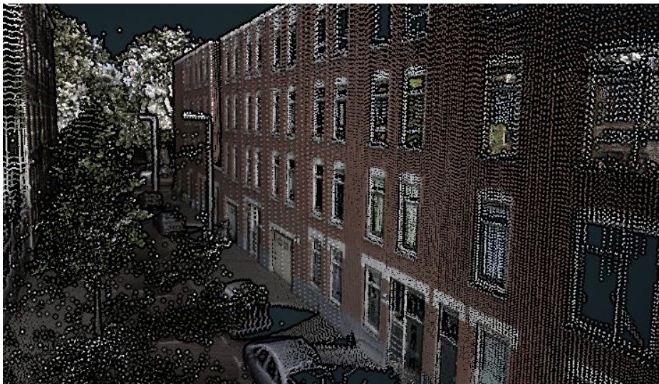
Figure 5.17: Example of the Noordereiland MLS dataset on street level (source: Gemeente Rotterdam / own work)
