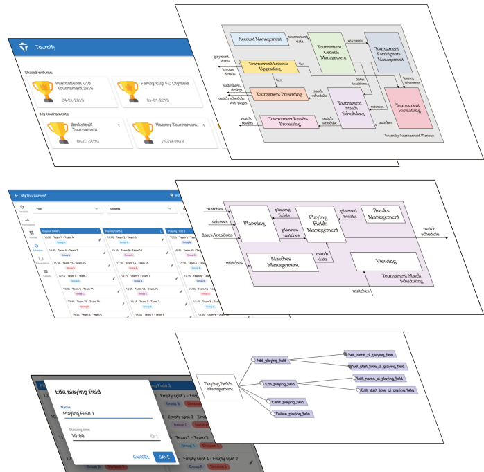
Fig. 5. Three-layered functional architecture of a web application, recovered based on the GUI.
