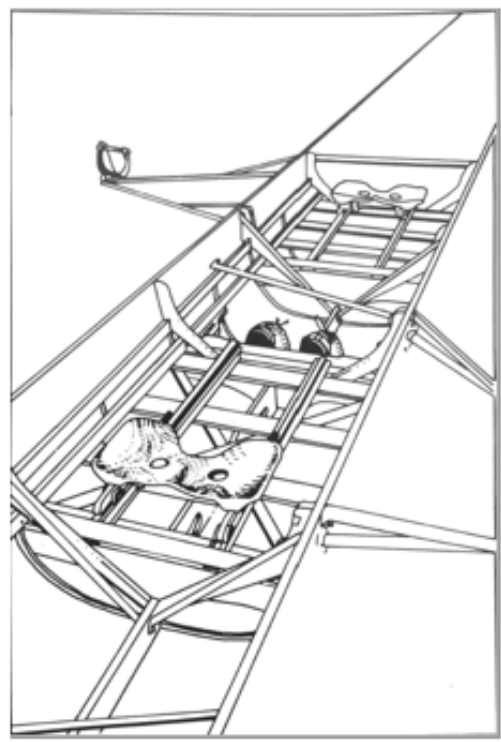
A detail of a wooden shell's construction, showing slide, stretchers, rigger, keelson and stringers.
