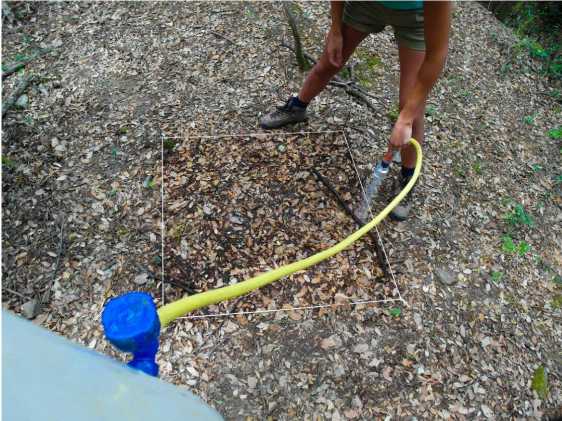
Figure 4-12. A 11mm rainfall event was simulated on a 1m 2 meter plot of in this case the dense matorral forest floor.
