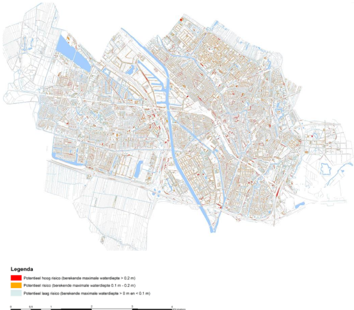
Figure 6 Potential inundation of Utrecht with precipitation amount of 60mm/h (Municipality of Utrecht, 2015)
