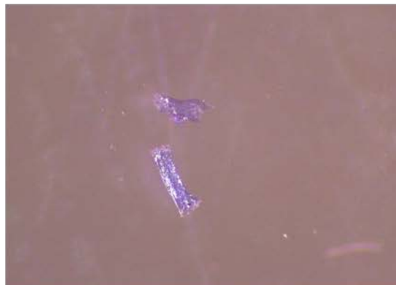
Sample: 5-10-2010-AMM-003_postFTIR Composition: Polyethylene / Polyethylene terephthalate
