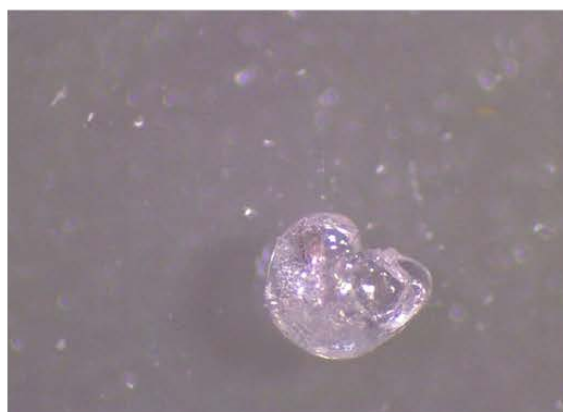
Sample: 2-2010-SPR-B008_a Composition: Polymethyl methacrylate
