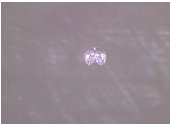
Sample: 7-09-2010-AMM-B007_a Composition: Polymethyl methacrylate
