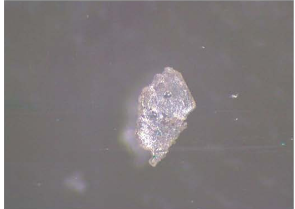
Sample: 5-11-2010-SPR-B001_b Composition: Polyethylene
