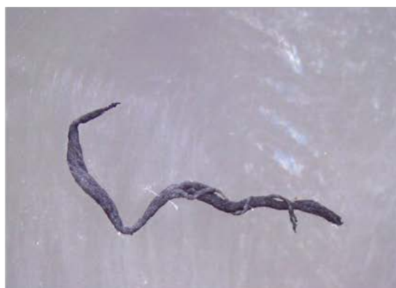
Sample: 3-03-2016-SPR-B004_b Composition: Polyethylene/Polypropylene copolymer
