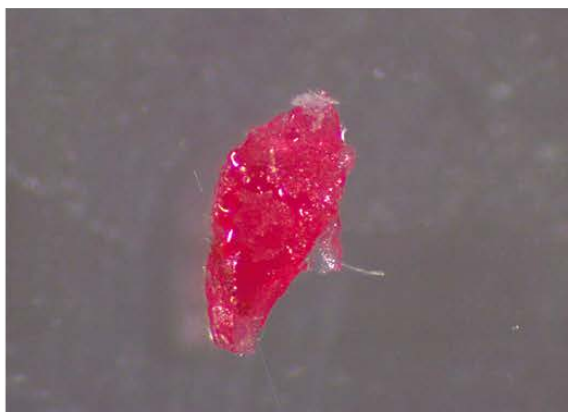
Sample: 1-03-2013-SPR-B001_a Composition: Polypropylene
