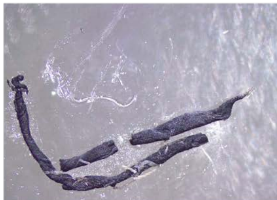
Sample: 3-02-2016-SPR-B002_b Composition: Polyethylene/Polypropylene copolymer
