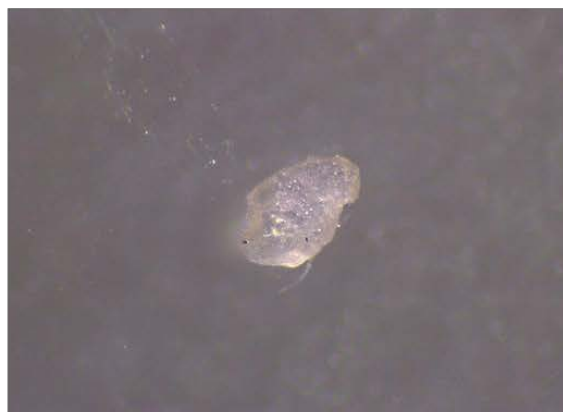
Sample: 1-03-2013-SPR-B001_b Composition: Polyethylene
