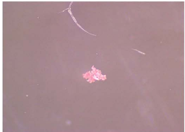
Sample: 7-09-2010-AMM_B004 Composition: Polybutylene terephthalate
