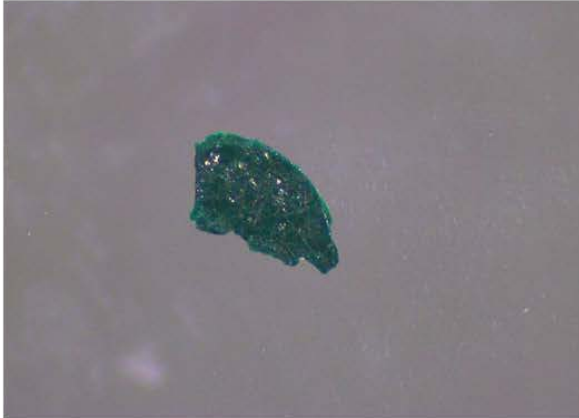
Sample: 5-11-2010-SPR-B001_a Composition: Polybutyl methacrylate
