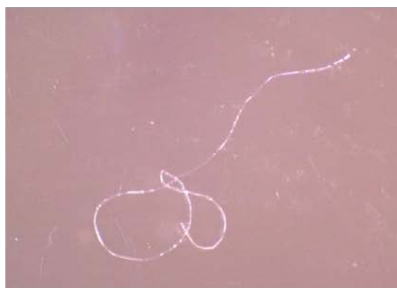
Sample: 7-09-2010-AMM-B007_b Composition: Polyethylene terephthalate
