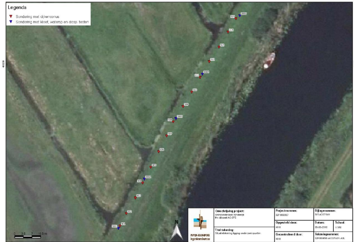
Figure A.4 Location AC 075 at the north dike of the drainage canal Achterwaterschap with the locations of the class 1+ cones (red points) and class 1 cones (blue points).
