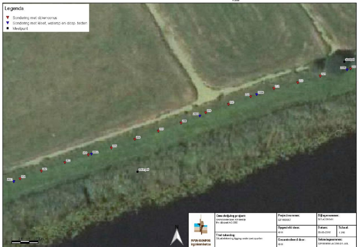
Figure A.5 Location AC 090 at the north dike of the drainage canal Achterwaterschap with the locations of the class 1+ cones (red points) and class 1 cones (blue points).
