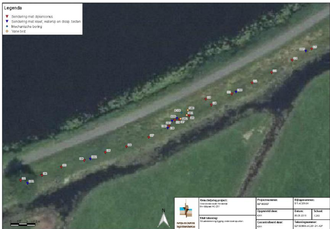
Figure A.3 Location Achterwaterschap at AC 251 near Alblasserdam with the locations of the class 1+ cones (red points) and class 1 cones (blue points).
