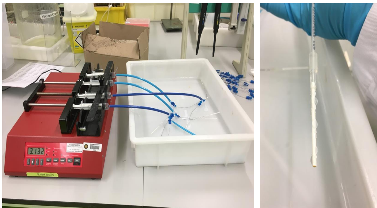
Figure 13: Left photo Rhizon cleaning setup from a test run in which the flow rate was reduced and a total of 8 rhizons were attached. Cleaning was done on 4 rhizons at a time connected to the 0.6 ml/min rate controlled pump. Right photo visual inspection of undamaged flow through rhizon filter.
