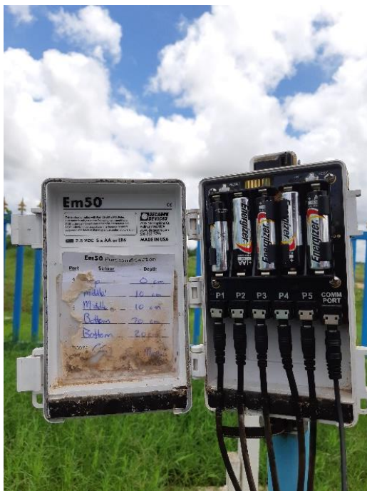
Figure 9: Data logger of nest 2 with 5 connected sensors. The com port is used for connection with a laptop.
