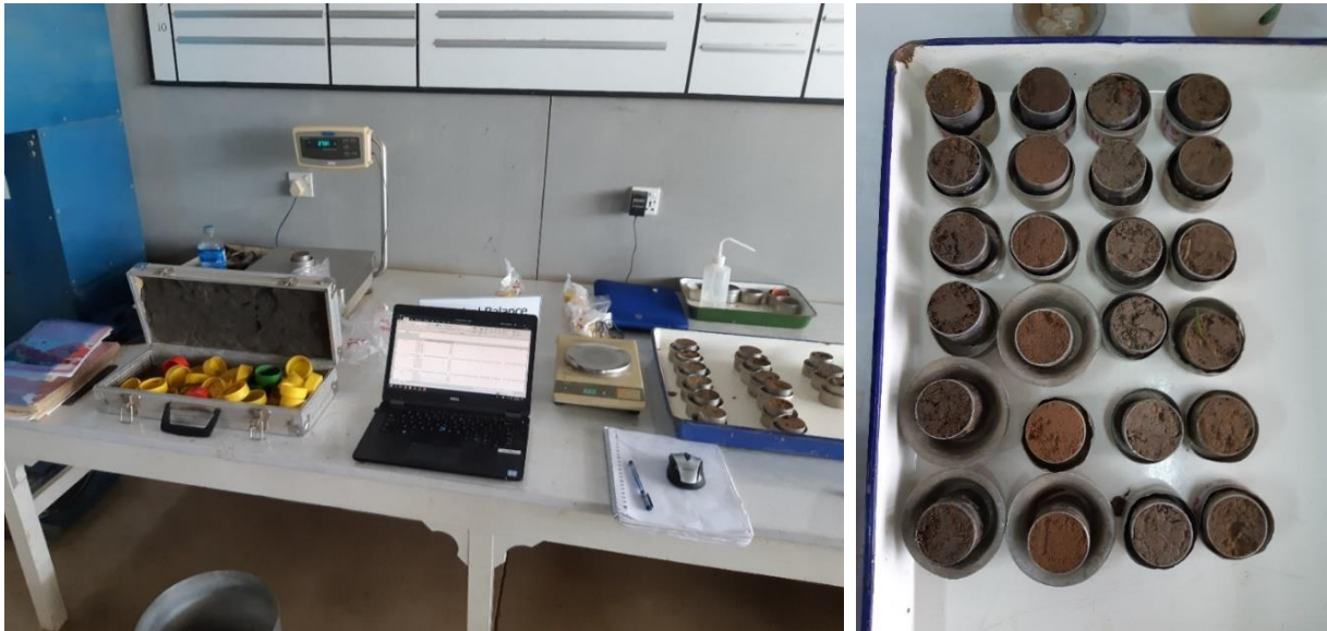
Figure 7: Weighing the samples and storing the data. Figure 8: The wet samples before going in the oven. Stacked columns from left to right: nest 1, nest 3, nest 4 and nest 5.
