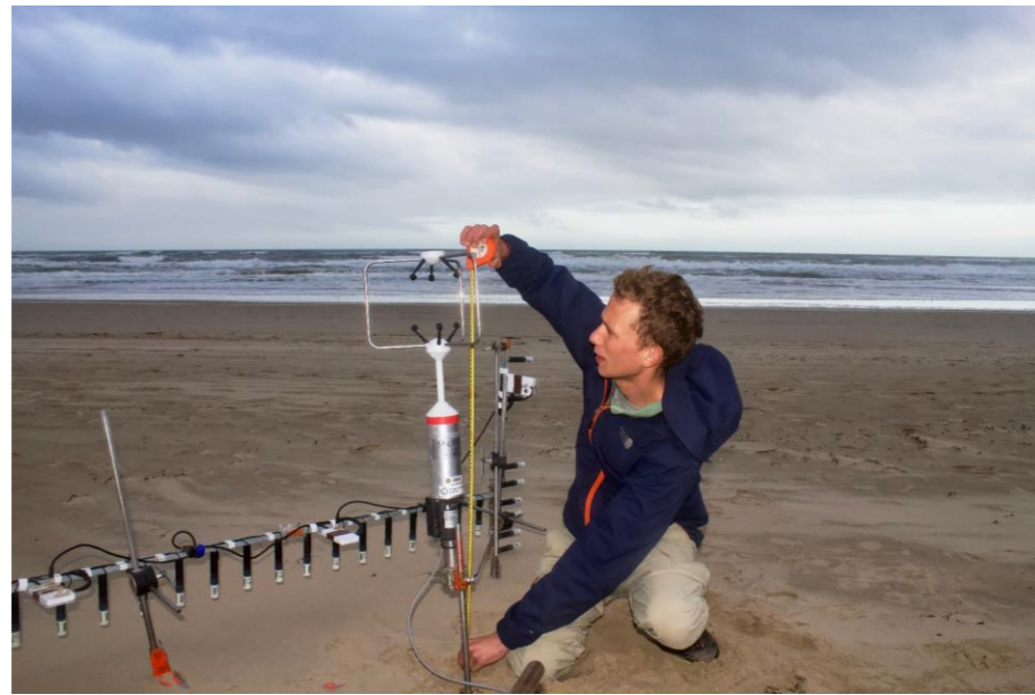
Figure 8.2. Setting up of equipment, adjusting g height of Sonic Anemometer before setting it level
