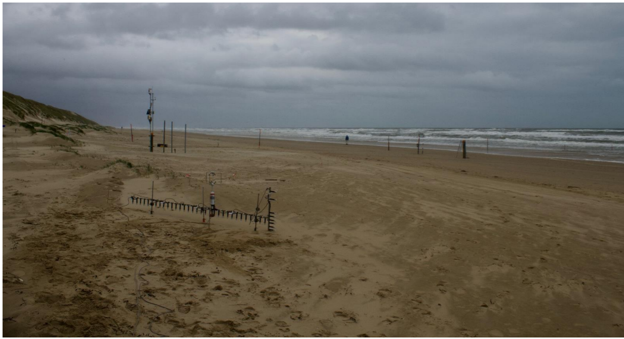
Figure 8.1 Impression study site with saldec and Sonic anemometer on the foreground. Other equipment in the background
