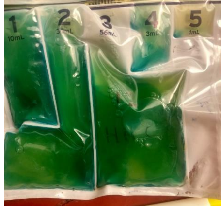
Figure 39: E. coli test in Malawi. All compartments have turned (partly) green, indicating a most probable number of coliform units/100 mL of >100.
