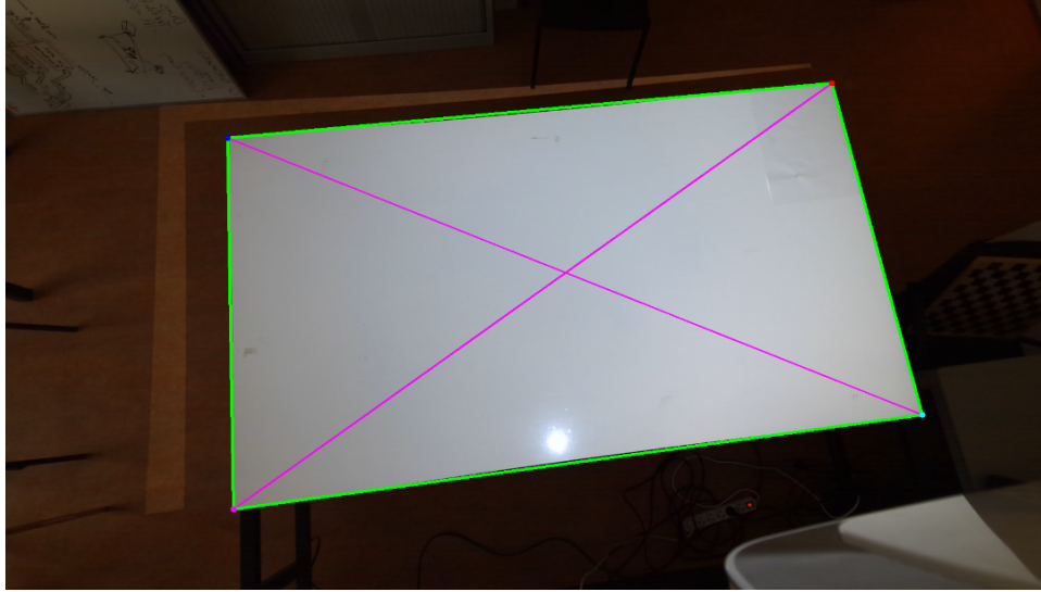
Figure 4.6: Calibration of color camera 3. Corner points found by using diagonals.
