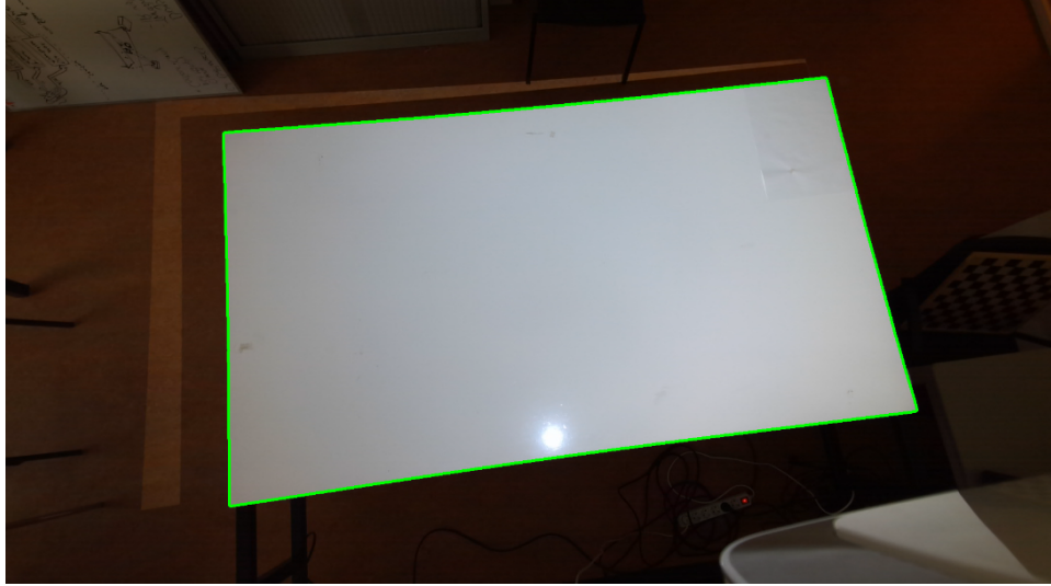
Figure 4.4: Calibration of color camera 1. Largest contour found by using Canny edge detection.
