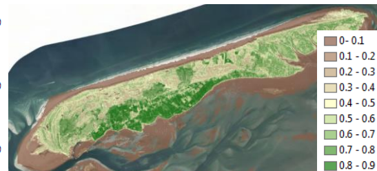
Figure 0-5 - Calculation of NDVI in GEE and an example of the result: NDVI index for Terschelling for 13-05-2000
