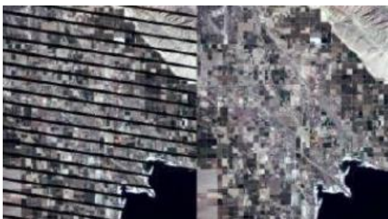
Figure 3-2 - Malfunction of the SLC causes scan lines to appear: left shows SLC-off and right is with the SLC-on (USGS, 2018b).
