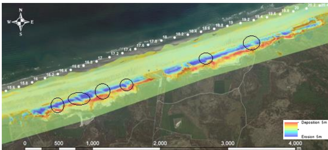
Figure 3-14 - Foredune remobilization after human interference, captured in an elevation difference map from airborne Lidar data (1997-2010) in Terschelling. Seven of eight blowout locations can be derived (black circles). Distance between white dots at the coastline is 200 m (Arens et al., 2013).
