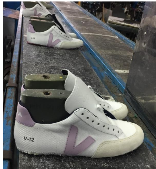
Figure 14: Upper with the shoe last. Source: VEJA, 2018.
