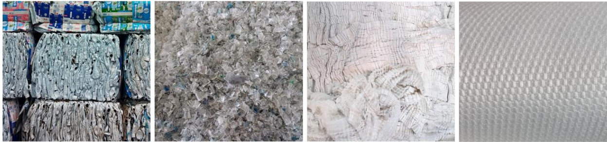
Figure 10: Stages of Recycled PET's life cycle, i.e. sorting of plastic bottles, PET flakes, polyester fibers and fabric. Source: VEJA, 2018.
