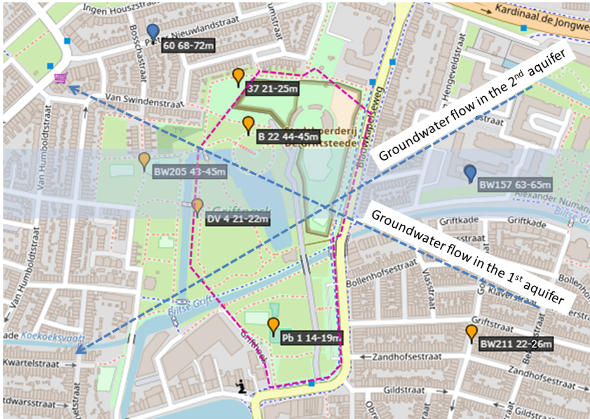
Figure 9: Location of the selected wells in and around the Griftpark. The yellow pinpoint represents the monitoring wells in the 1st aquifer and the blue, the 2nd aquifer. The pink dashed line indicates the presence of the slurry wall. The blue shaded area shows where the patches with incomplete clay layer (aquitard) can be present. The blue arrows visualize the direction of the groundwater flow in the 1st and 2nd aquifer (not inside the slurry wall).
