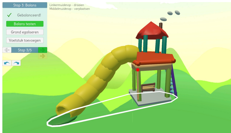
FIGURE 4.6: Balance analysis. The convex hull of the floor vertices is colored white. The center of mass is the red dot. If the center of mass (projected to the floor) is within the convex hull, the model is balanced.
