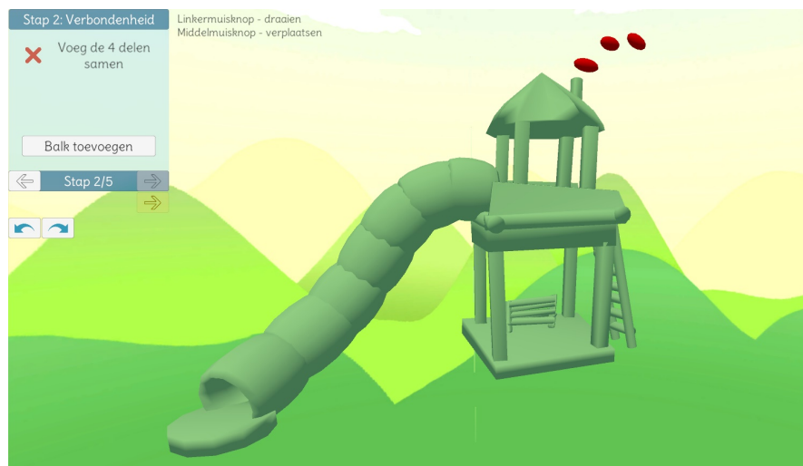
FIGURE 4.5: Connectedness analysis. Disconnected pieces are colored red.
