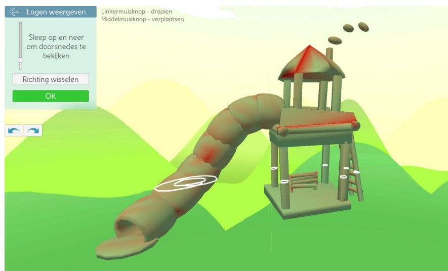
FIGURE 4.7: Strength analysis. Thin pieces are colored red. A cross section is colored white.
