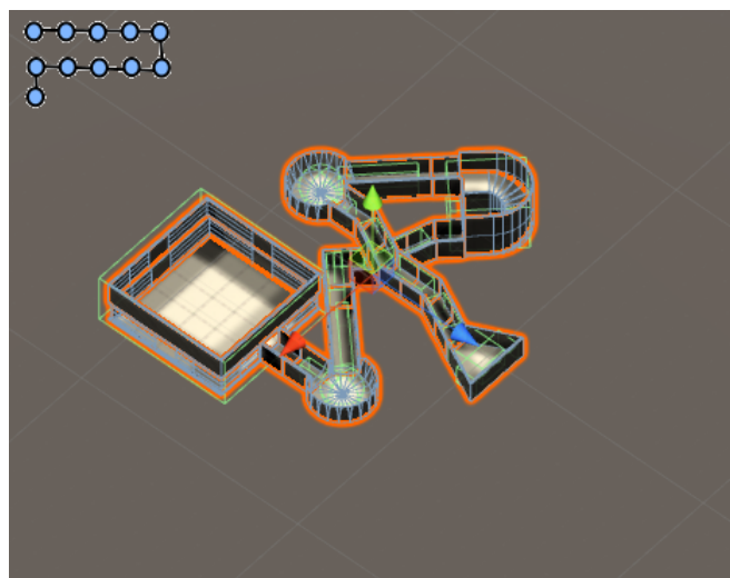
FIGURE C.2: A generation output with module set 3 for a linear graph with 11 nodes.
