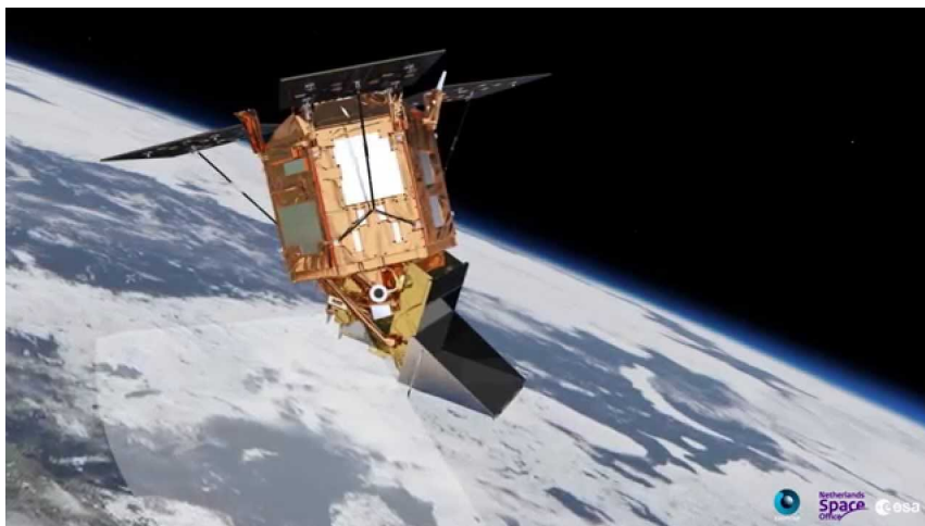
Figure 1.2: Illustration of Sentinel-5 Precursor satellite with one single payload on board, TROPOMI (Source: ESA/ATG medialab).
