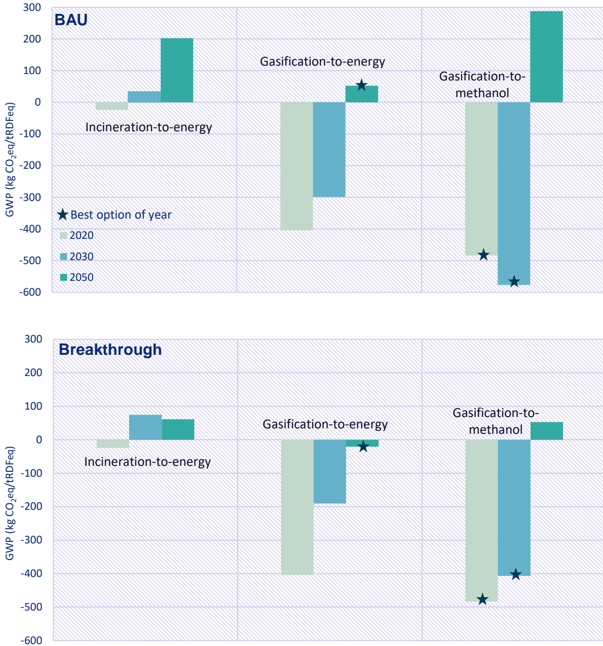
Figure 18. Net GWP (RDF product compared to reference product) of each waste treatment from 2020 to 2050 including production and use phase of the BAU Scenario (top) and Breakthrough Scenario (bottom). The star indicates the most favorable waste treatment option for that year.
