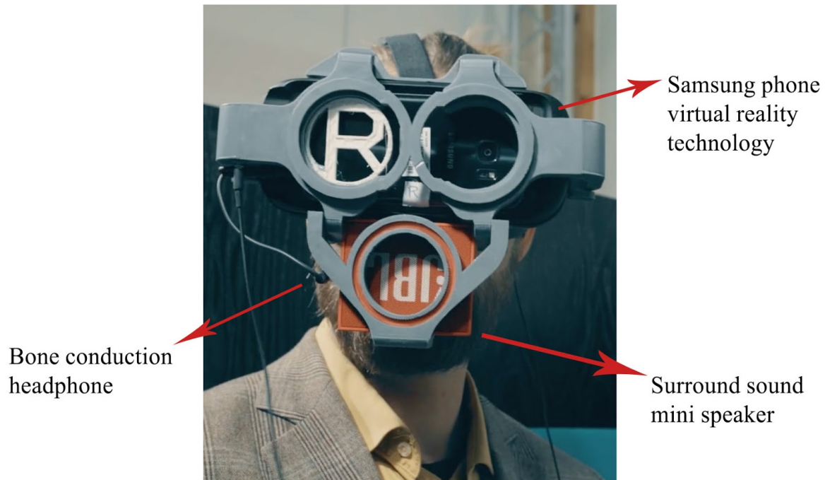
Figure 5: Here I have added my own annotations to an image of the Anyways headset. Indicating where the technology is positioned within the 3D printed plastic mould (PIPS:lab 2017)
