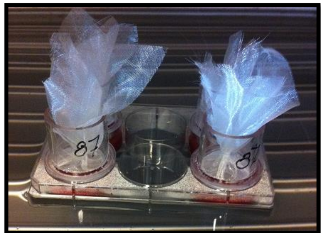
Fig. 4 The completely assembled feeding units as used in the water bath
