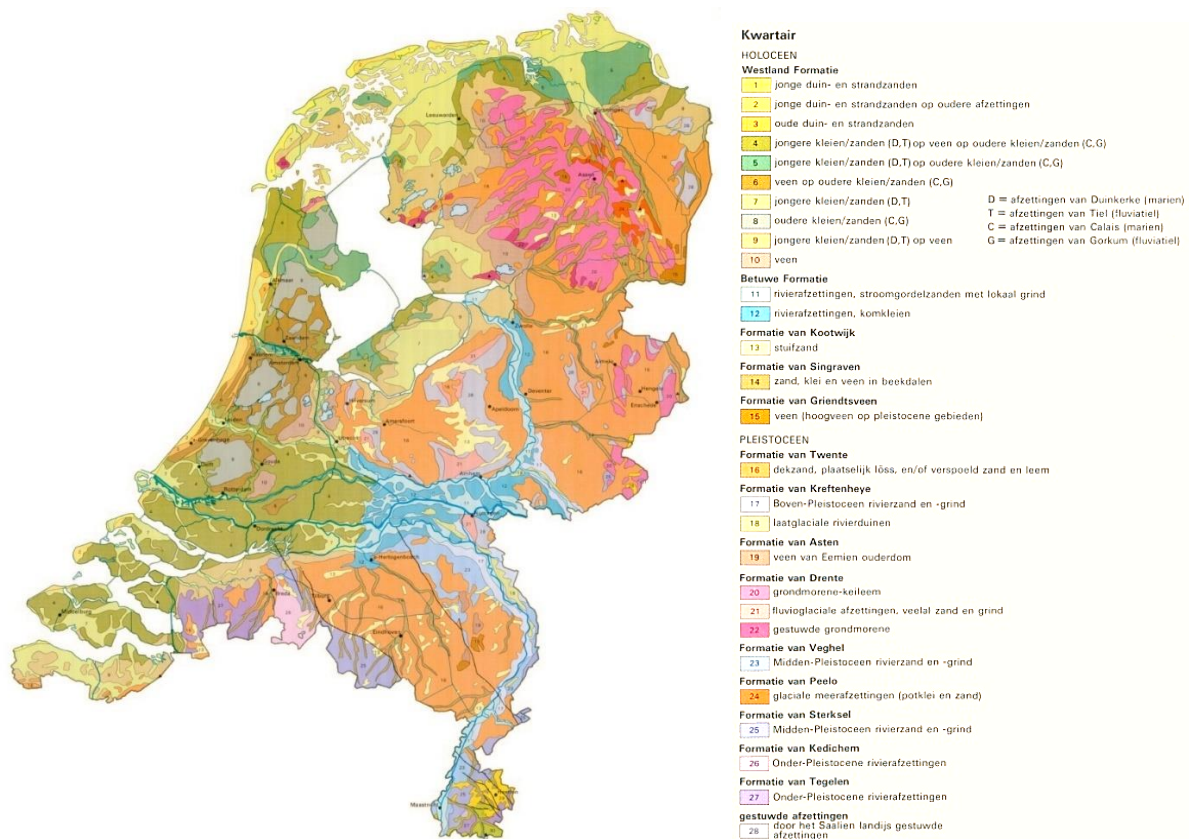
Figure 3.1 Geological map of the Netherlands. To show older formations, the cover sands deposited in the Weichselian are only displayed if the layer is more than 2 m thick ("Atlas van Nederland, deel 13: Geologie, 1985," 2001).
