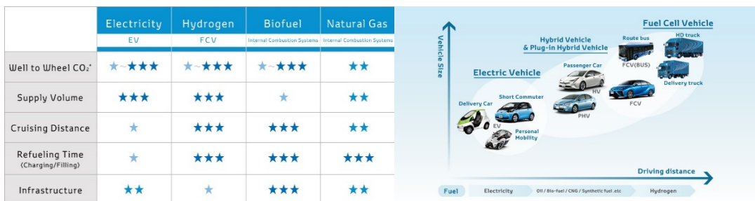
Figure 5 Characteristics of gasoline-alternative fuels evaluated by Toyota
