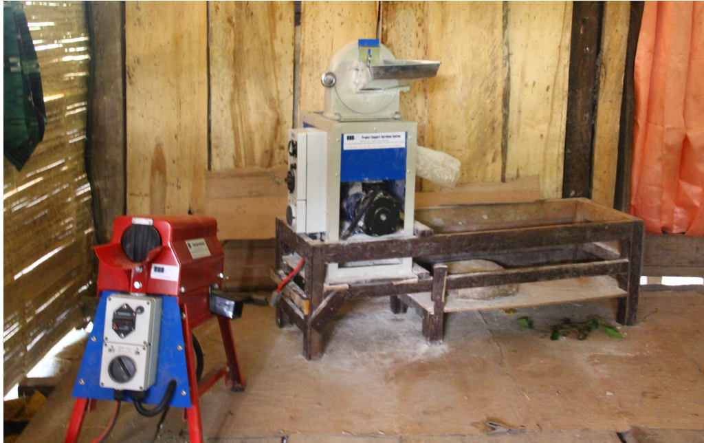
The PV agro-processing machines. The red machine is a corn sheller and the grey one grinds the corn into flour.
