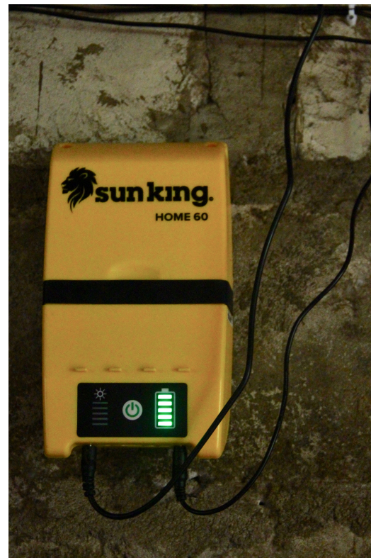
A solar home system. A small PV pane (see cover photo) lies on the roof, the battery is shown on the right and one of the three lamps lighting up the house on the left.
