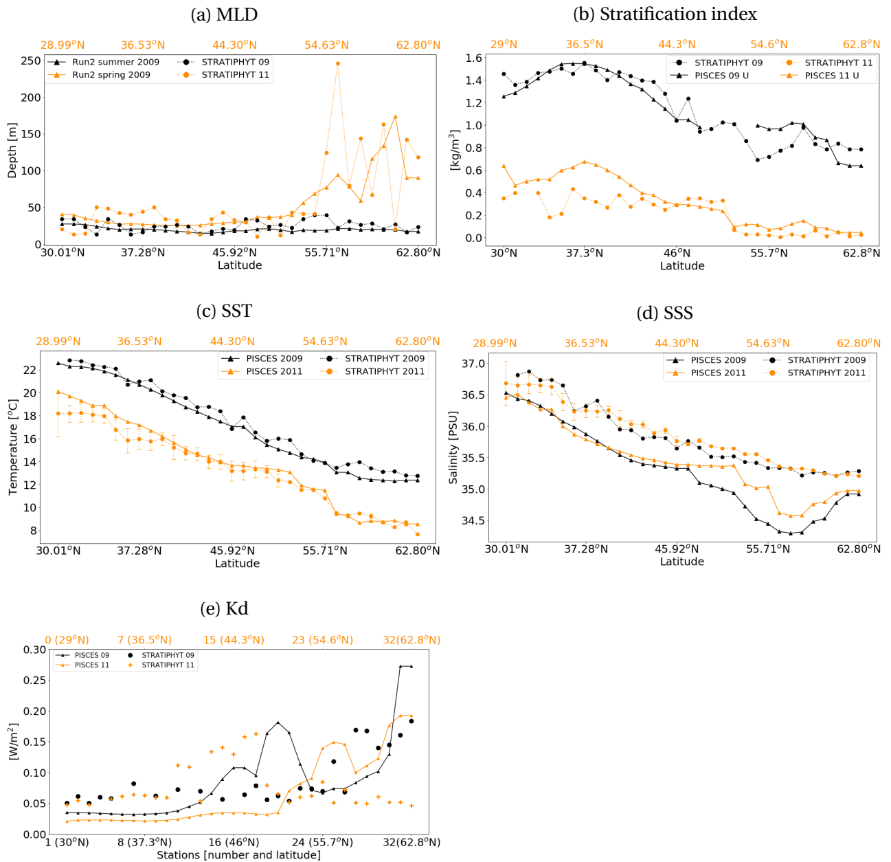
Figure 4.1: Physical parameters (MLD, SI, SST, SSS and Kd) as measured by STRATIPHYT cruises (orange dots for 2011 and black for 2009) and model results as April-May (orange triangles) and July-August (black triangles) averages along the transect shown in Fig. 3.1. Standard deviation is plotted as errorbars around the STRATIPHYT curves (orange and black color). Latitude is along the x-axis with orange (for 2011) and black color (for 2009).
