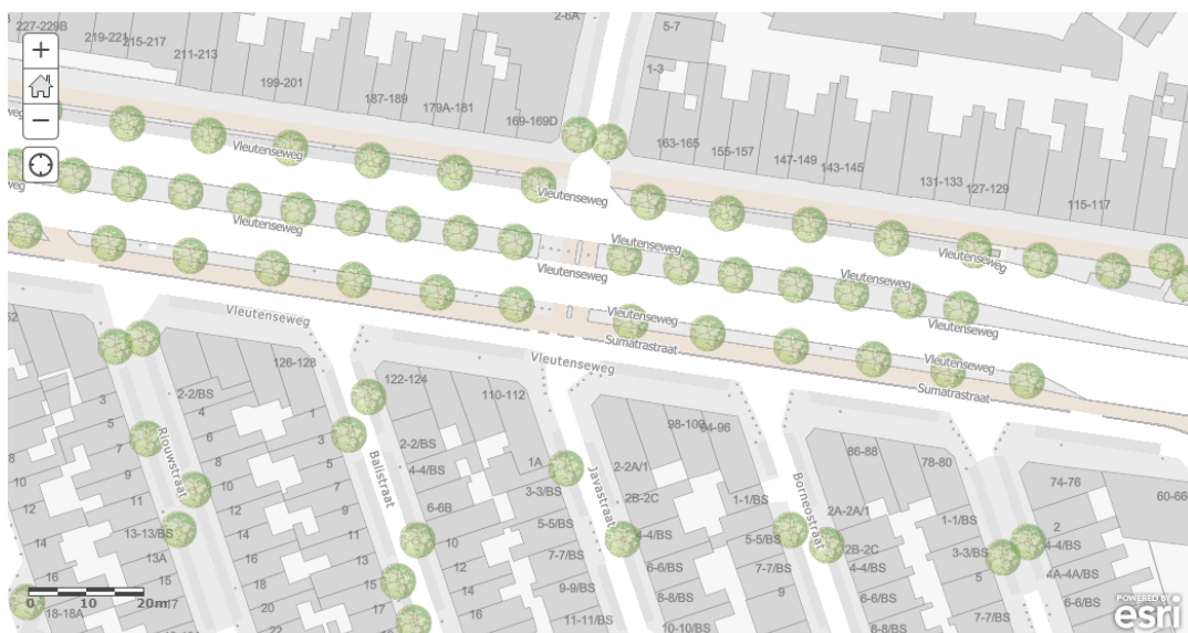
FIGURE 7.2: ESRI Topo RD Vector Tiles in Beta; repetition of labels issue (PDOK, 2018b)
