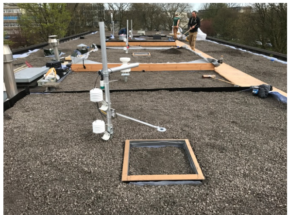
Figure A3 Placement of the substrate and the setups. The square in the middle is the lysimeter with climatic measurements next to it.
