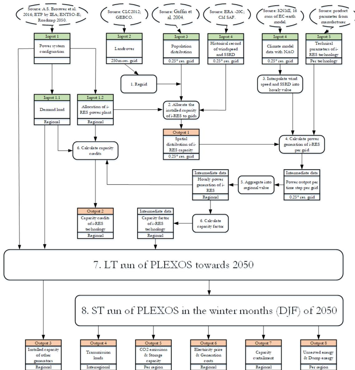
Figure 3. Overview of the input data, operation procedure and the outputs.
