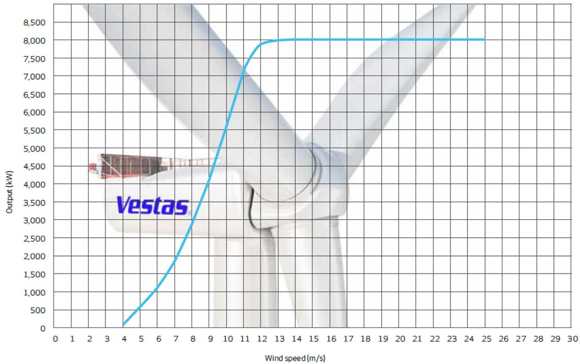
Figure D-2. Power curve of offshore wind turbine (Vestas 2011).
