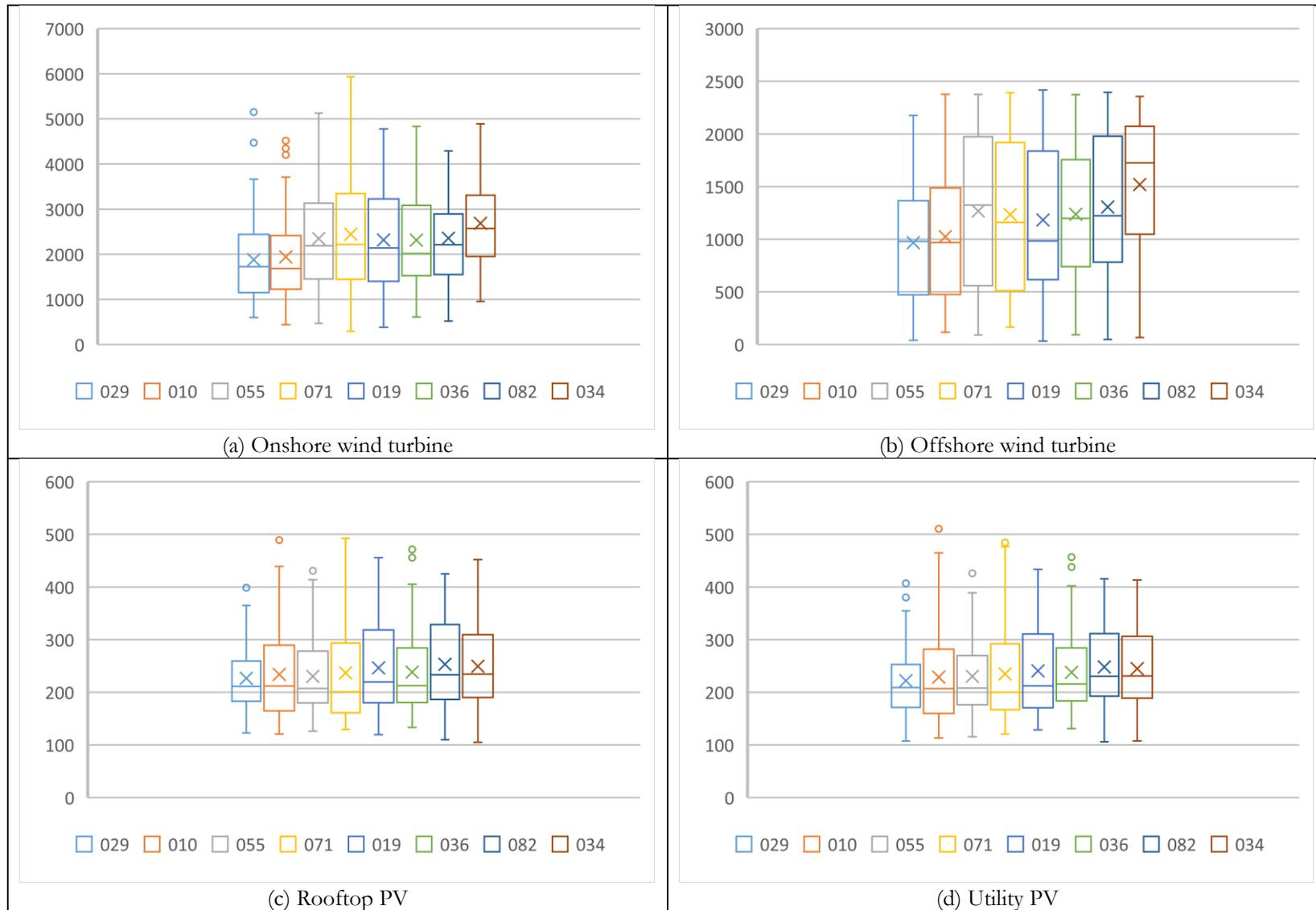
Figure 8. Distribution of daily power generation [GWh] per iRES in winter months (DJF). The box plots represent total electricity output available per day per iRES technology. A bar in the box shows the median. A cross in the box shows the mean. In each plot, boxes of weather years are ordered with increasing NAO index as shown below.
