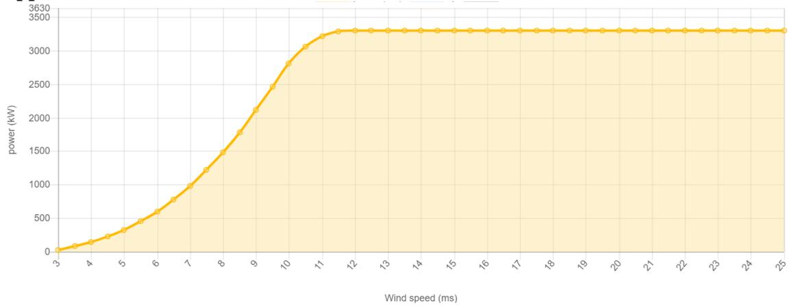
Figure D-1. Power curve of onshore wind turbine.
