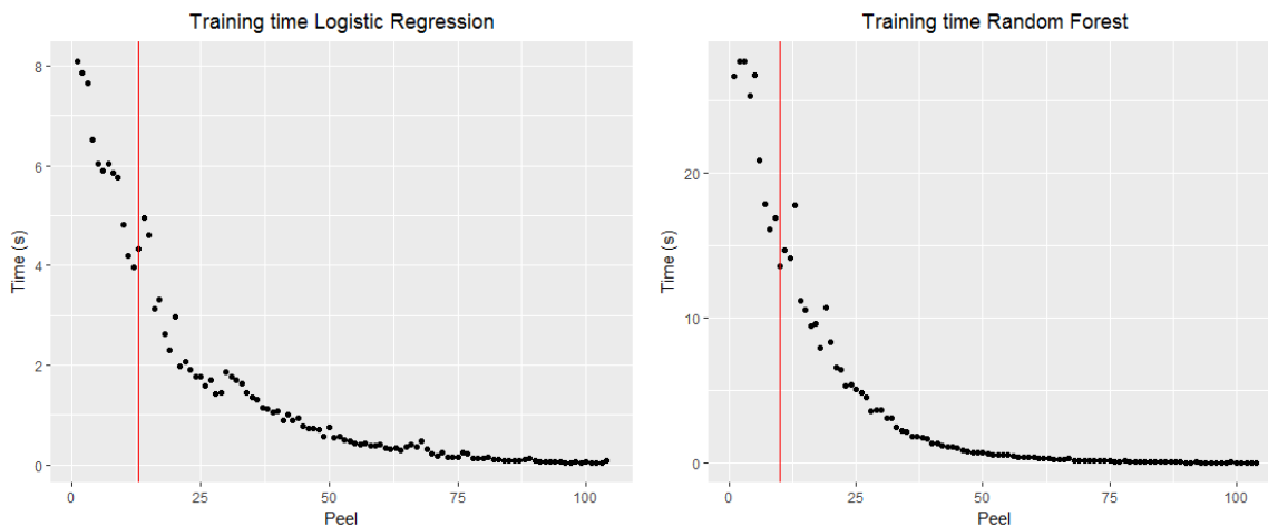
Figure 4.4: Time required for training a classifier on each subbox resulting from a peel according to the process from figure 4.3. Red lines indicate when the process passed the half of the total time.
