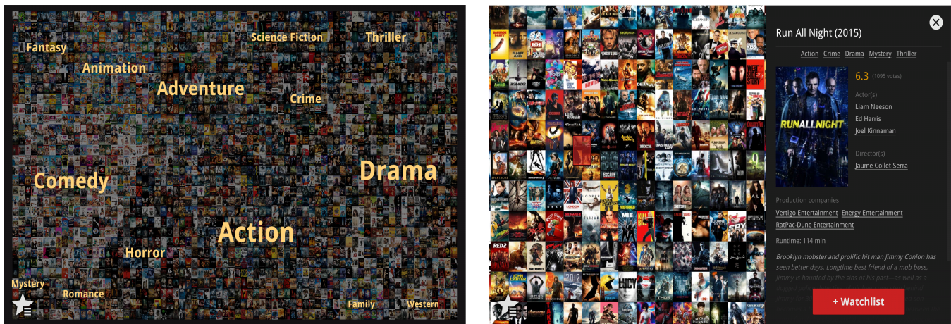
Figure 1: The MovieWall interface. On the left side, one can see the interface completely zoomed out, which also serves as the starting point. The headers show the centers of each cluster, as well as the genres used. On the right, a view of the MovieWall zoomed-in, with the details panel open. Headers disappear as the user zooms in. All movie posters were downloaded from www.themoviedb.org and used under the fair usage policy.
