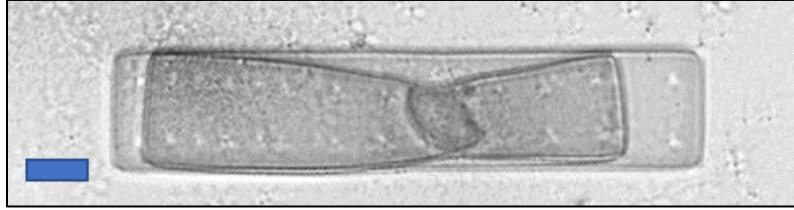
Figure 4) Overlay of a 220\mu\text{m} \times 50\mu\text{m} crawler in maximally shrunken and expanded states, scale bar = 25\mu\text{m} .
